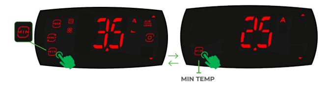
2 Press MIN button to display min temperature. Press min again to return to unlocked screen.
