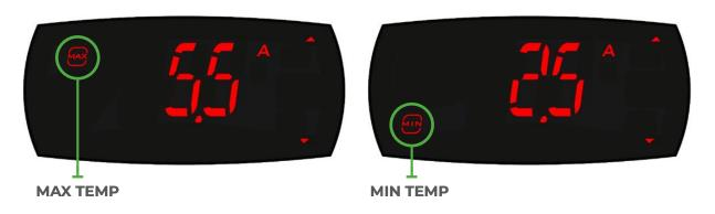
3 The controller will display MAX or MIN depending on the selection.
