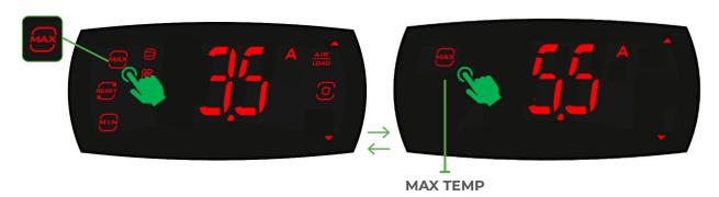
1 Press MAX button to display max temperature. Press max again to return to unlocked screen.
