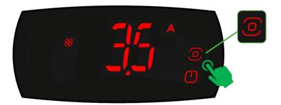
1 Press and hold the navigation button for 3 seconds
